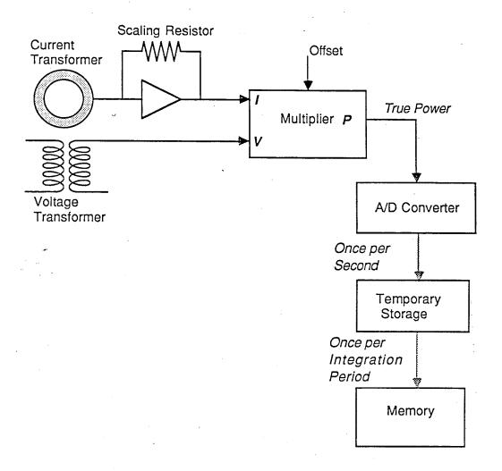
FIGURE 1. Schematic of a Typical Sensor Channel
